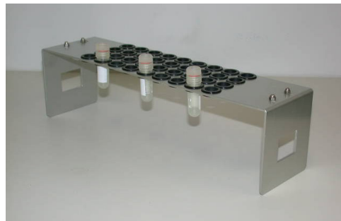
Figure 2: 1.5 (2) mL tube rack TR-4002 (Micro tube mixer MT-400 supplied rack; TOMY Seiko)
